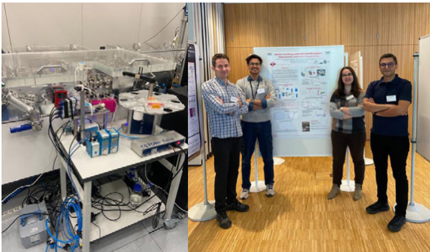
Left: Home-built automated sample handling system with modulated sample exchange. Right: Microfluidics team presenting at the ATTOWORLD-alumni meeting (from left to right: Dr. Igor Kukhtevich, Akash Singh, Dr. Elisa Lambert, Amaj Chamankar). Images: FRIS-team
