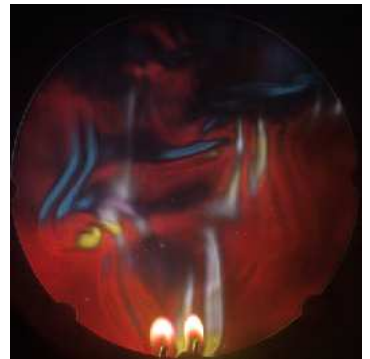
The picture shows a candle in a single-mirror schlieren photographic apparatus, which uses four color filters instead of a razor blade to separate the refracted light. This makes the horizontal and vertical separation of the light visible. This allows you to do more than just separate "dense air from less dense air", but also to make the 3-dimensional form visible
